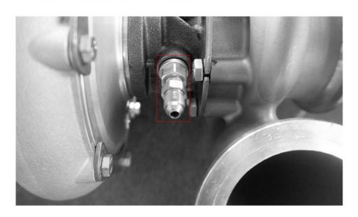
44.install turbo oil outlet lfange, flange seal, flange whasher, and flange fastening bolts (torque 20nm)
