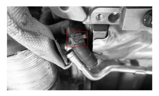
20.Remove the bolts on Turbo Water Return Line with T30 Socket
