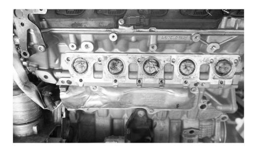
28.install the twin thread Studs supplied by JDY on the Exhaust Manifold
