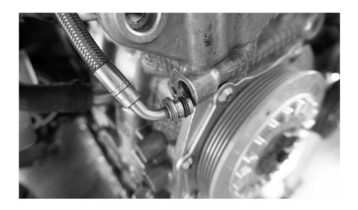
14.Remove the Bolts on the OEM Water Pipe from Cylinder Block with M8 Socket
