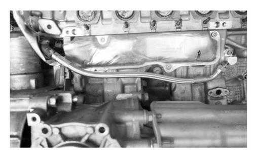
36.Install the JDY Flange to Cylinder Block using OEM Bolts with Torque applied at 10NM
