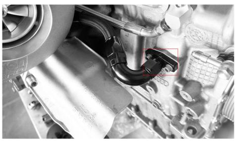
47.Intall the JDY Oil Return Line with 14mm Wrench (install Oil Return Line angled 90°, AN4 Fitting toTurbocharger, install Oil Return Line angled 45° to the engine Block)"
