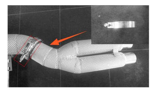
59:Fix the intake aluminum pipe onto the compressor cover inlet using clamp bolts supplied by JDY with H4 Socket
