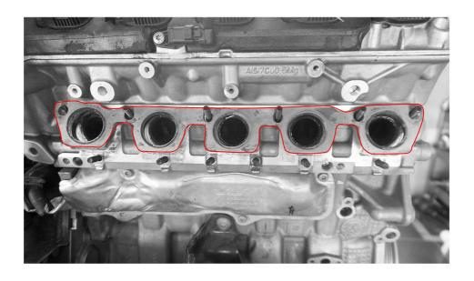
30.install the JDY Heat Shield with the botls supplied by JDY using H5 Socket with Torque applied at 10NM
