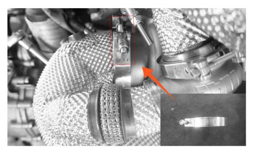
56:Fasten the MVR and Downpipe Clamp Bolts with H4 Socket (Adjusting both of the turbo and downpipe in every direction possible to the stage where there's no clearance in between. Then fasten all the bolts on turbo, downpipe and MVR clamp with torque applied at 10NM)
