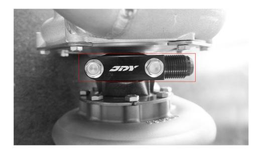
45:Fasten the bolts on JDY Intake manifold and Turbo Clamp with 13mm Socket (Make sure the turbo's put at the right place adjustable. With everything being set in place, then it's time to fasten the clamp bolts with torque applied at 15NM)
