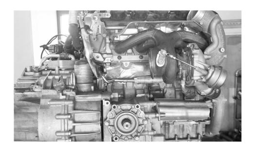
4.Remove the Bolts on OEM EGR(Exhaust Gas Recirculation) Pipe with T30 Socket
