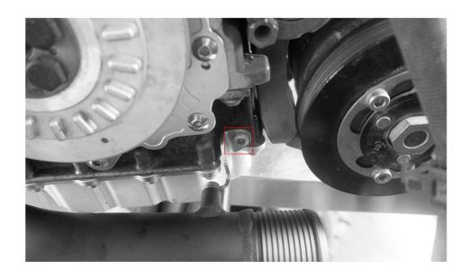
54.Fasten the bolts on the MVR and Exhaust Manifold with H4 Socket (Make sure the MVR's put at the right place adjustable. With everything being set in place, then it's time to fasten the clamp bolts with torque applied at 10NM)
