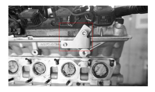
31.by using M8 socket, install the coolant return flange on the engine block, with torque of 10nm
