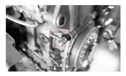
38.Install the JDY oil inlet Flange supplied to Cylinder Block and install the JDY Flange washer using OEM Bolts with Torque supplied at 10NM
