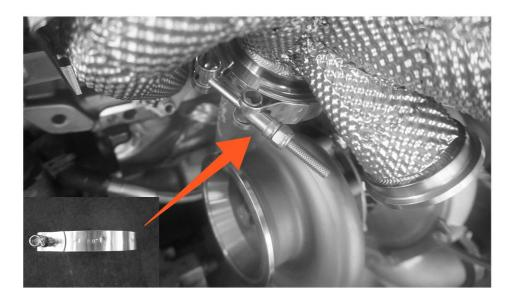
46.Intall the JDY Oil Return Line with Wrench (Oil Return Line angled  $60^\circ$  on the Turbo, , Oil Return Line angled  $120^\circ$  on the block"
