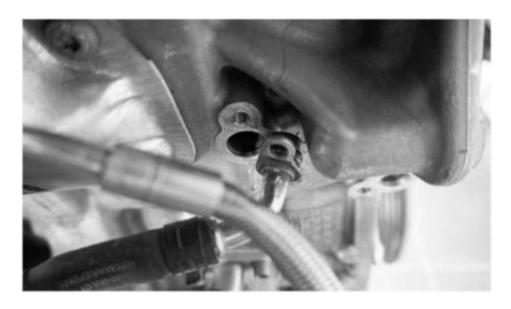
16.Remove the Bolts on the OEM Turbo Oil Return Line with M8 Socket
