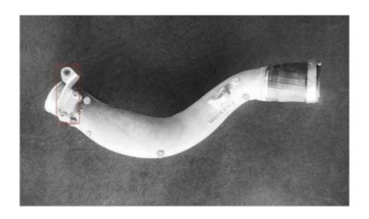
50.Install the OEM Bracket on the JDY Turbo Charge Aluminum Pipe with T30 Socket
