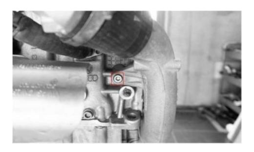
10.Remove the OEM Charge Scilicon Pipe Clamp with 7mm Socket
