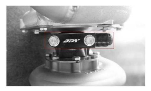
45:Fasten the bolts on JDY Intake manifold and Turbo Clamp with 13mm Socket (Make sure the turbo's put at the right place adjustable. With everything being set in place, then fasten the clamp bolts with torque applied at 15NM)
