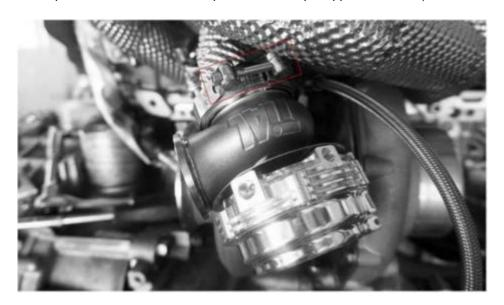
55:Fasten the bolts on J DY Intake manifold and Turbo Clamp with 13mm Socket (Make sure the downpipe's put at the right place adjustable. With everything being set in place, then it's time to fasten the clamp bolts with torque applied at 15NM)
