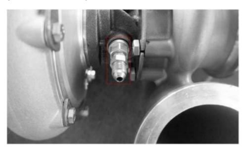
44.install turbo oil outlet Ifange, flange seal, flange whasher, and flange fastening bolts (torque 20nm)
