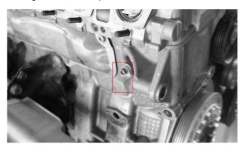
32.Install the JDY 1/8NPT To AN6 Fitting on the Flange installed from previous step with 16mm Socket
