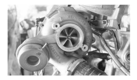
8.Remove the Bolts on the OEM Charge Aluminum Pipe Bracket with T30 Socket
