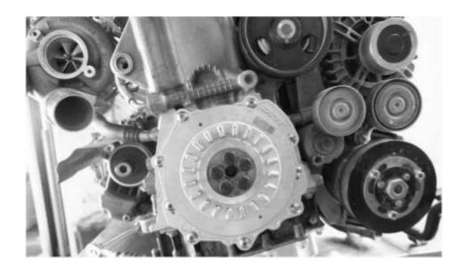
12.Remove the Botls on the OEM Oil Inlet Pipe from Cylinder Block with M8 Socket
