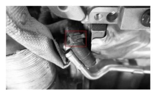
20.Remove the bolts on Turbo Coolant Return Line with T30 Socket
