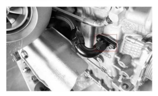
47.Intall the JDY Oil Return Line with 14mm Wrench (install Oil Return Line angled  $90_\circ$ , AN4 Fitting toTurbocharger, install Oil Return Line angled  $45_\circ$  to the engine Block)"
