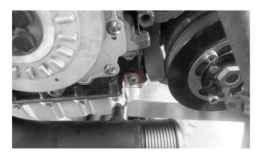
54.Fasten the bolts on the MVR and Exhaust Manifold with H4 Socket (Make sure the MVR's put at the right place adjustable. With everything being set in place, then fasten the clamp bolts with torque applied at 10NM)
