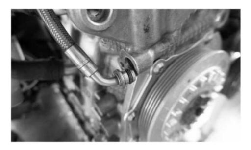
14.Remove the Bolts on the OEM Coolant Pipe from Cylinder Block with M8 Socket
