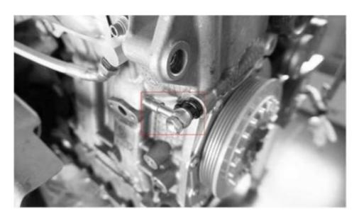
38.Install the JDY oil inlet Flange supplied to Cylinder Block and install the JDY Flange washer using OEM Bolts with Torque applied at 10NM
