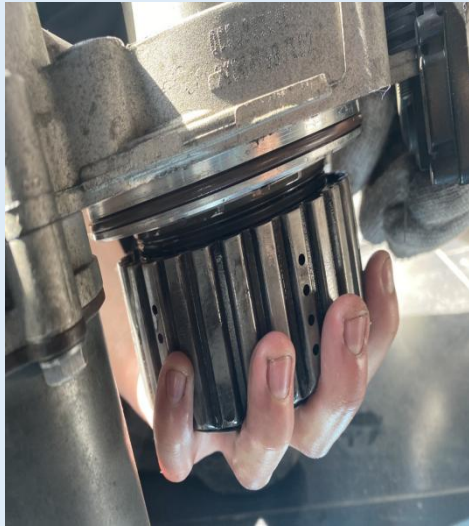
Install the clutch drum upwards into the end cover of the four-wheel drive clutch, and screw in the hexagonal nut
