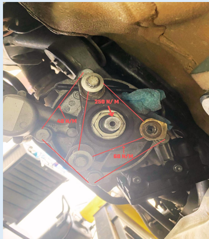
Install the clutch drum upwards into the end cover of the four-wheel drive clutch, and screw in the hexagonal nut
