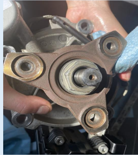
Install the clutch drum upwards into the end cover of the four-wheel drive clutch, and screw in the hexagonal nut
