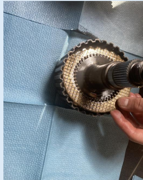
2.first step is to place the friction plate.
