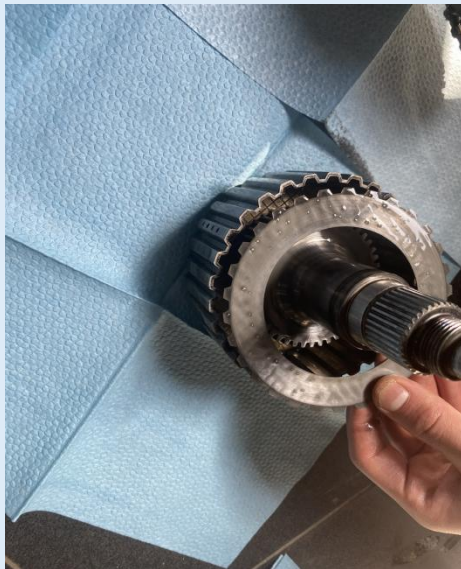
The next step is to place the steel plate then followed by the serial.
