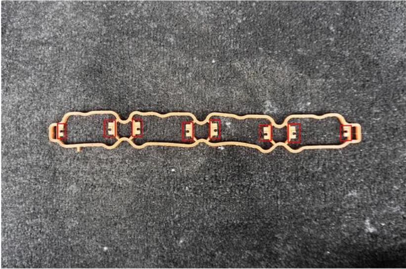
Cut the emphasized part of the gasket out and Install it on lower half of JDY intake manifold
