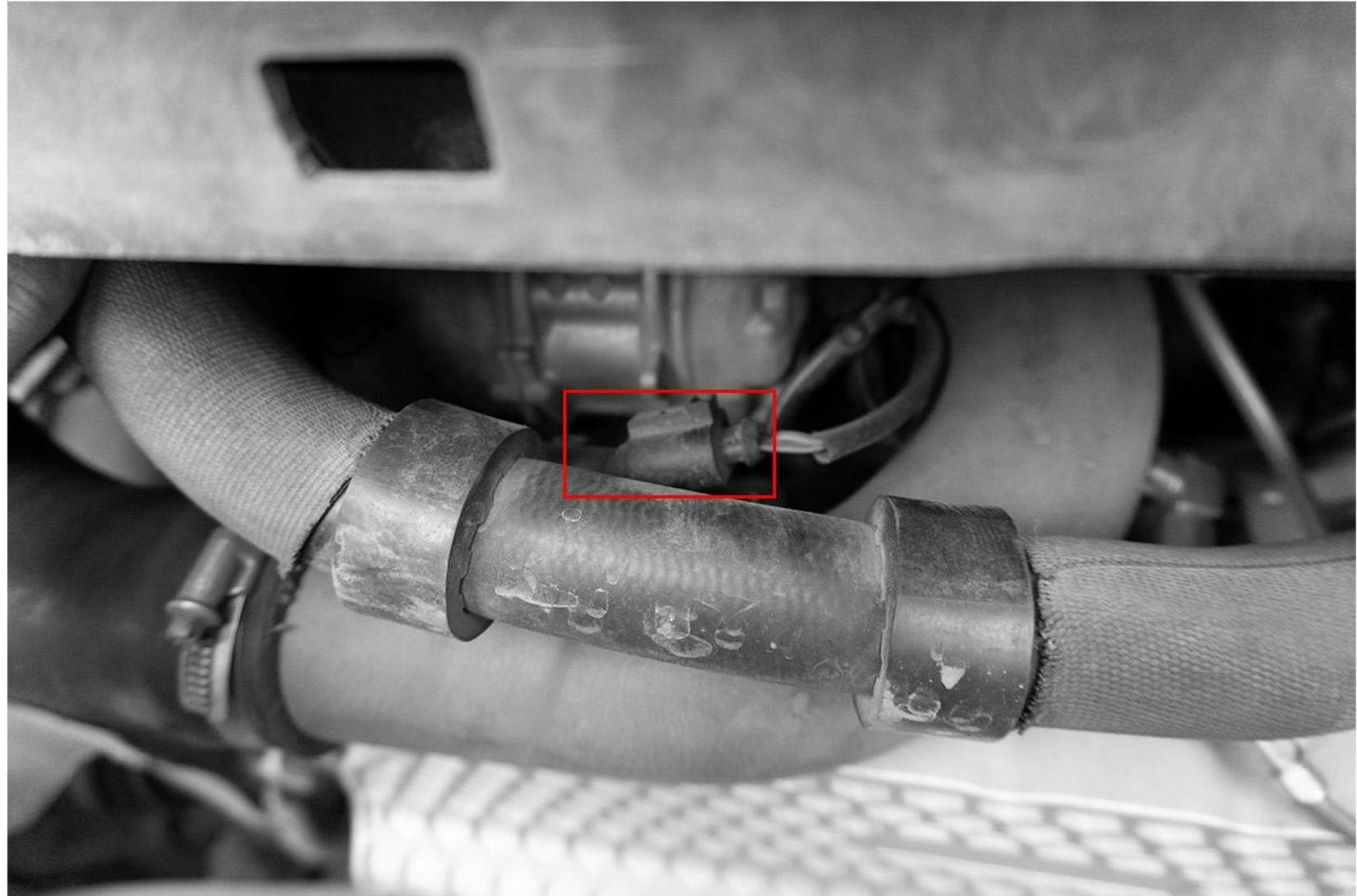
Disconnect the plug of boost pressure sensor
