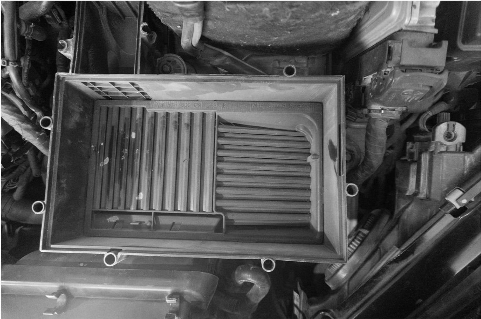
Remove the bolts on outlet pipe using T30 socket
