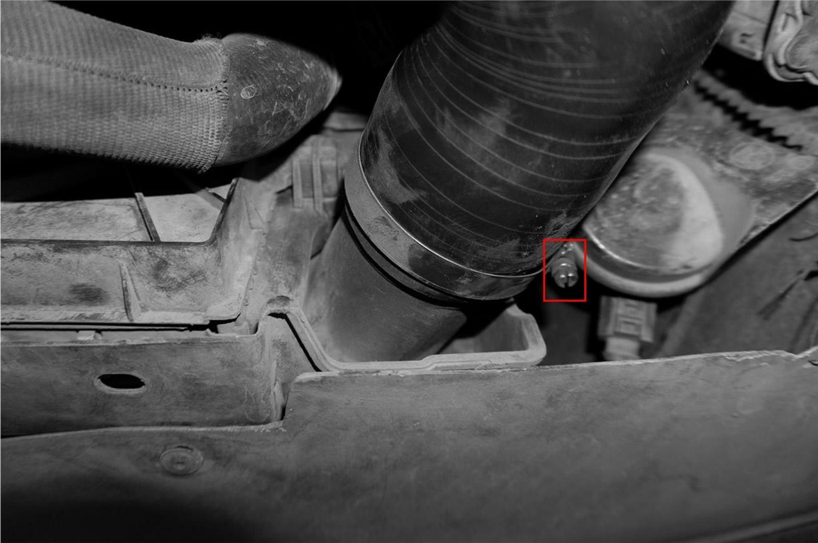
Fasten the bolts on the iron pipe alongside exhaust valve with T30 socket
