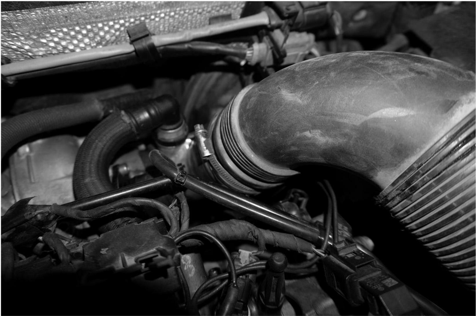
Fasten the bolts on air filter cap with
