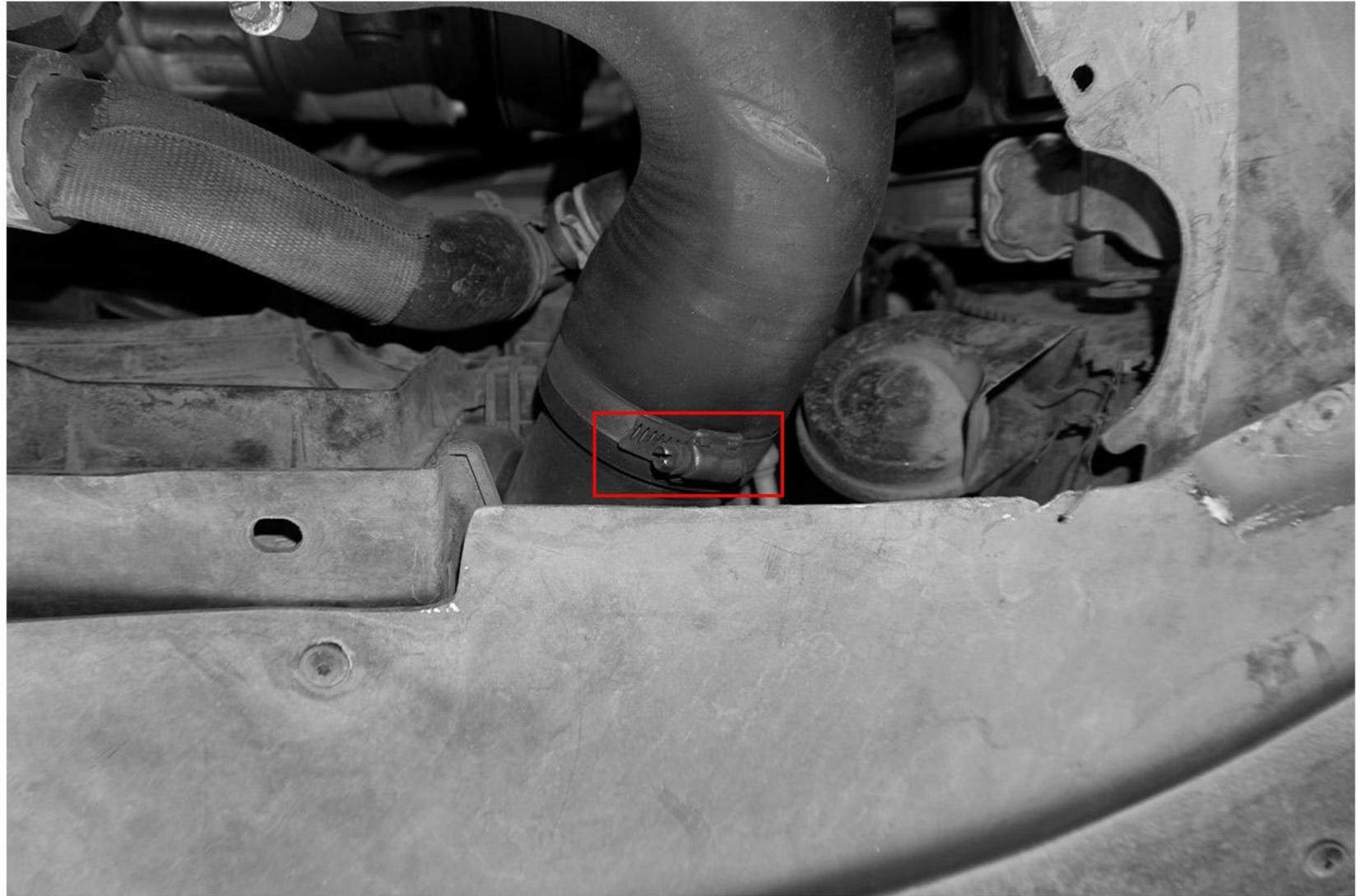
Disconnect the plug of boost pressure sensor
