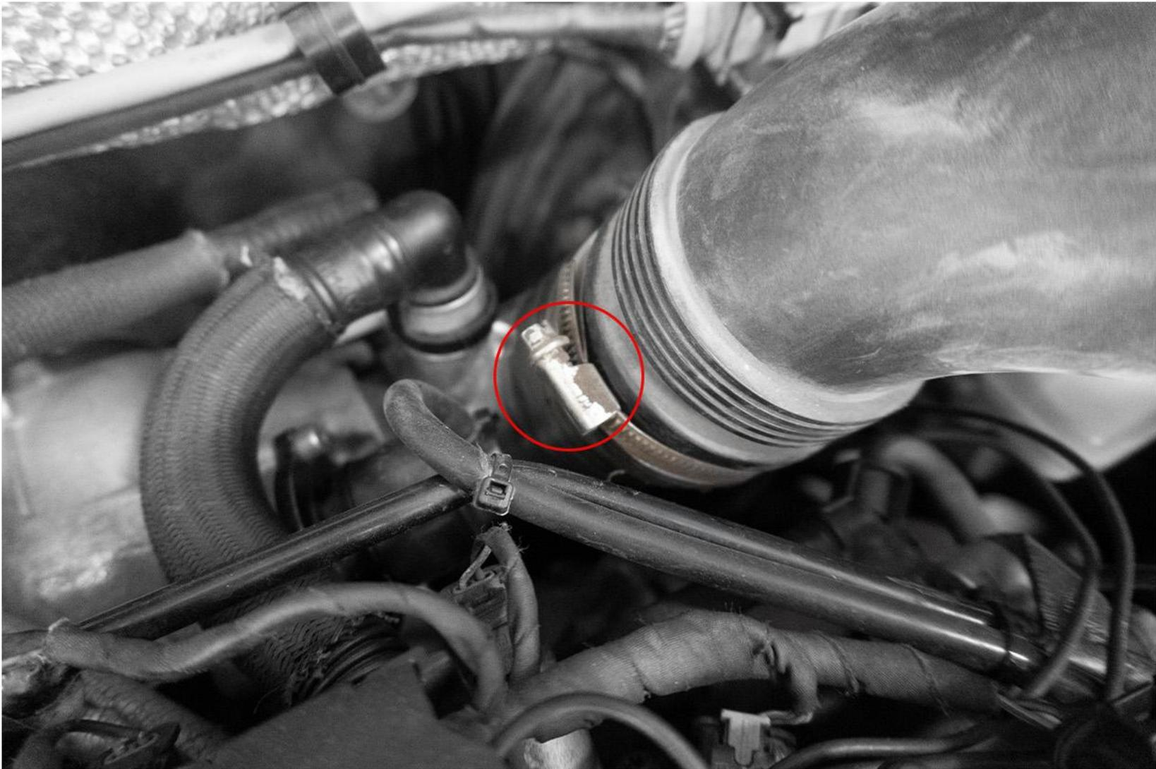
Remove the bolts on air filter cap with T25 socket
