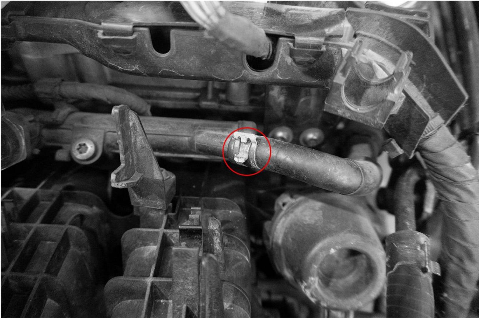
Remove the bolts on fuel rail with T30 socket
