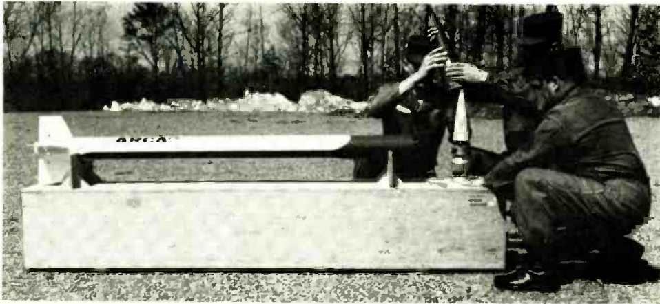
Army-developed rocket-borne radiosonde is loaded into the nose cone of a 77-pound rocket for its trip 40 miles into the atmosphere. After separation from the rocket, the radiosonde parachutes slowly to earth, transmitting weather information to earth.
