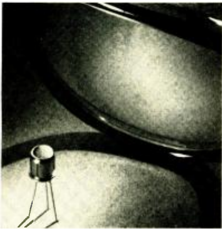
This tunnel diode is a low-cost G-E ZJ-56 germanium unit that will be of interest to amateurs and experimenters. Two of the leads shown are connected to the anode.
