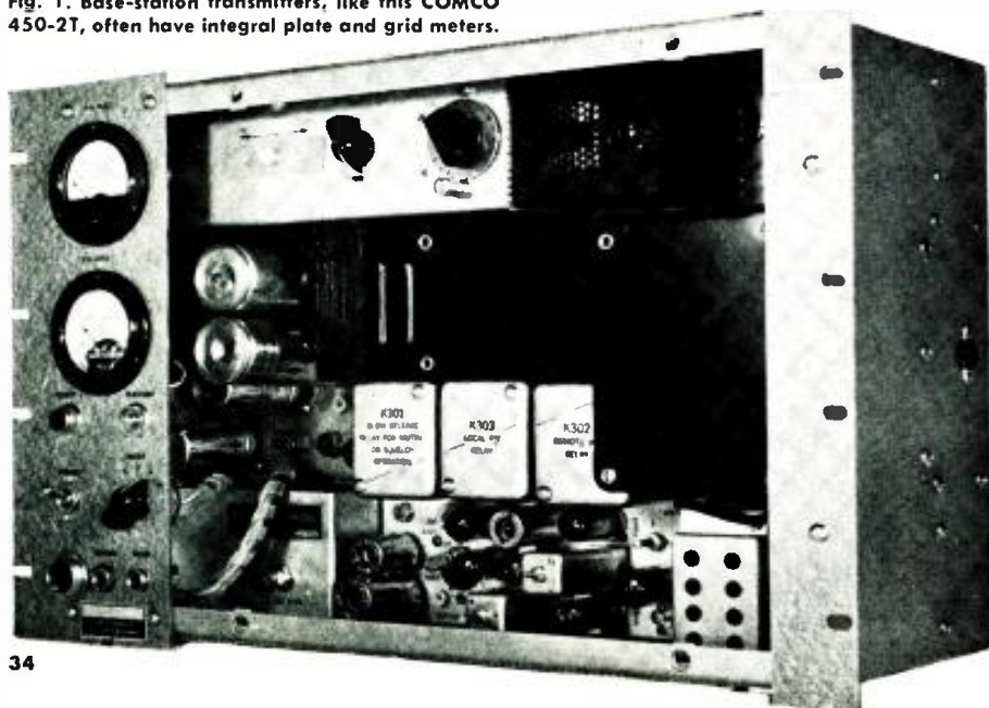
Fig. 1. Base-station transmitters, like this COMCO 450-2T, often have integral plate and grid meters.
