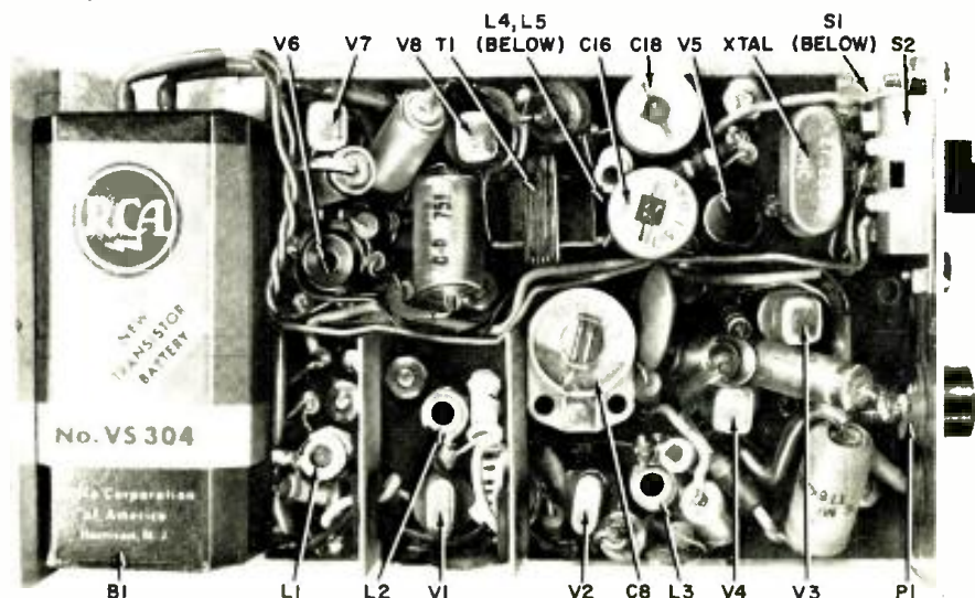
Top view of the chassis board showing very compact arrangement of components.
