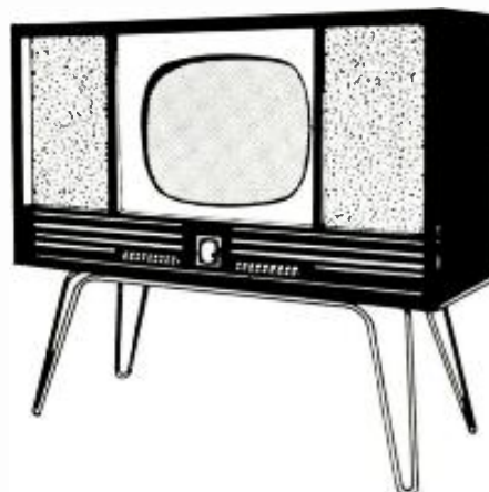
A new deluxe Soviet TV set with a 23-inch screen, 21 tubes and 19 diodes, 7 speakers, remote control, and FM broadcast reception.
