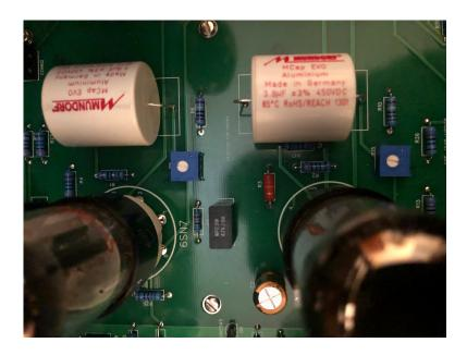
Turning clockwise will increase the gain, turning counter-clockwise will decrease the gain.
