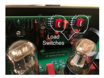
Only required set up on the MC board are The load settings for your particular cartridge, the Moving Coil head-amp is only required for low output moving coil cartridges >2.5mV, make sure that both switches at the back of the unit, the input switch and board switch are in the MC position
