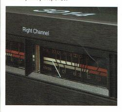
Meters on the Tandberg TCD 3014 indicate the signal after this record equalization has been applied. Therefore, they monitor the signal being recorded on the tape, not the signal coming into the record amplifier as most other recorders do. As all Tandberg cassette meters in the past, these are set to the now industry standard of 0 dB = 250 nWb/meter.
