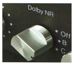
Dolby C includes improved circuitry which offers substantial improvement in signal-to-noise plus better high frequency overload capabilities. Dolby C in conjunction with Actilinear II and Dyneq achieves an outstanding musical signal free of annoying background hiss.
