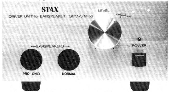
The SRM-1/MK-2 Professional has two output sockets; one for the SR-Lambda Professional (labeled "PRO ONLY") and the other for conventional earspeakers (labeled "NORMAL").
