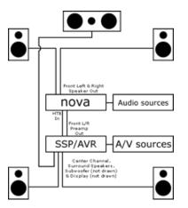
Connect Line-level (RCA style) front left and right outputs from the SSP or AVR to the AUX-1/HTB input on the nova.
