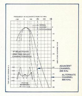
phase) is essential for low distortion FM reception. The MR 78 tuner uses linear phase filters at NORMAL and NARROW positions of the SELECTIVITY switch settings.
