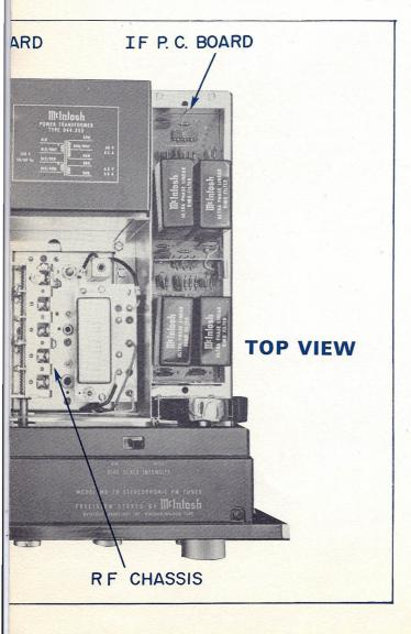
The linear-phase filter has flat time delay in its passband region. Any error in time delay causes FM distortion. All other IF filters have delay distortion, as much as 100%. The MR 78 filter has less than 1.0% delay distortion from antenna input to discriminator output.
