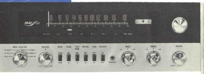
**HEADPHONE**—The headphone jack is for use with low impedance headphones. With the switch in the SPEAKER OFF position the loudspeakers will turn off when you insert your headphone jack. With the switch in the SPEAKER ON position the loudspeakers will remain in the system.
