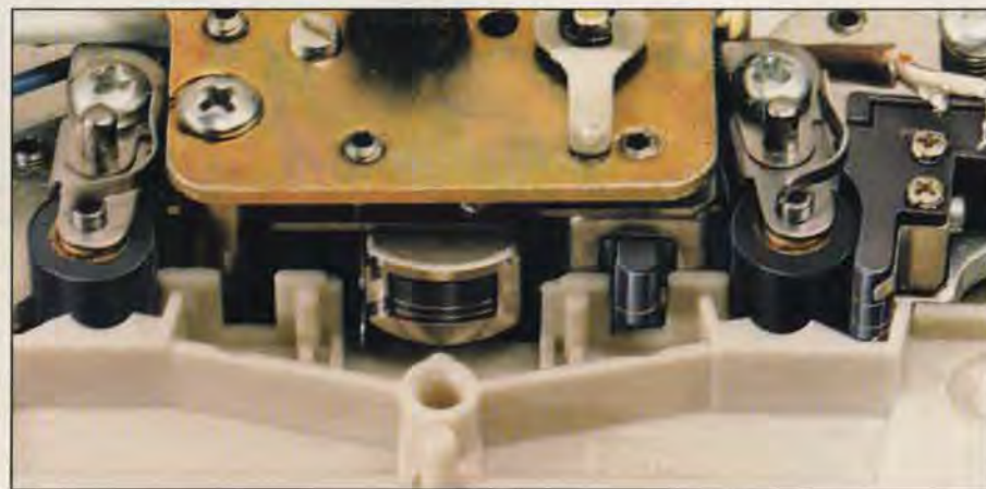
The problem of fitting three separate heads and dual capstans into the tape openings of the standard cassette is completely solved in the TCD 340 A design.
