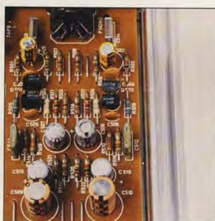
Phono signals are connected directly to a separate RIAA equalizer circuit.
