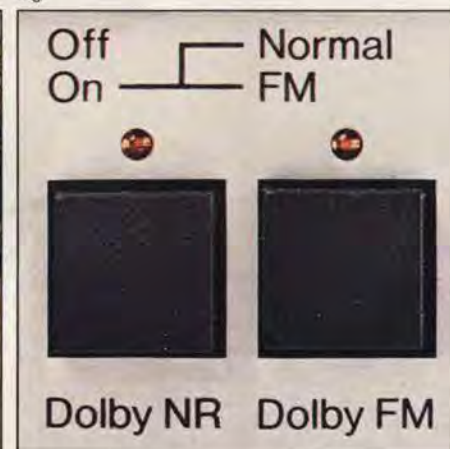
Separate record and playback Dolby circuits permit true record/playback comparison. Dolby FM stereo broadcasts can be decoded with or without recording.
