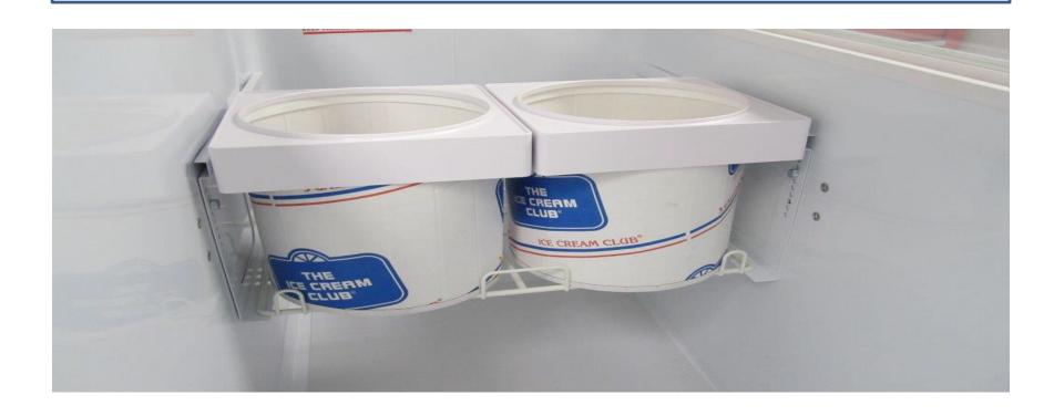
THE VIEW BELOW SHOWS TWO ICE CREAM CONTAINERS WITH CAN SKIRTS INSTALLED AND PLACED CORRECTLY ON SUPPORT RACK
