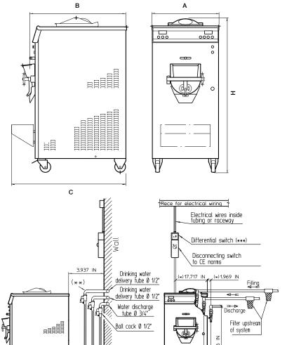
(\*) Even if the machine models vary, the water and electricity connection positions are always the same, i.e. on the LEFT side of the machine.
