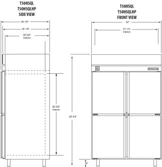
Cabinet designed for optimum performance in air-conditioned area at 70°F to 75°F ambient temperature and 50% to 55% relative humidity.
