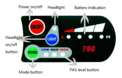
There are three buttons on the 790 display. Including power switch, mode button and headlight switch. In the following description, the switch button is replaced with the text "ON/OFF". The mode button is replaced by the text "MODE", and the headlight switch key is replaced by the text "LIGHT".
