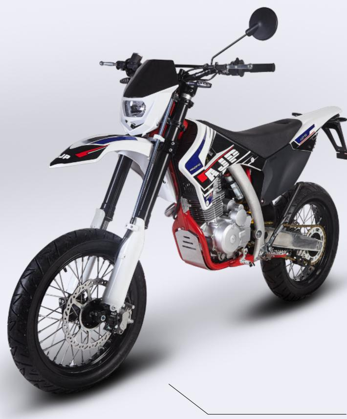
BRAKTEC dual piston caliper with Ø260mm front disc and single piston caliper with Ø220mm rear disc
