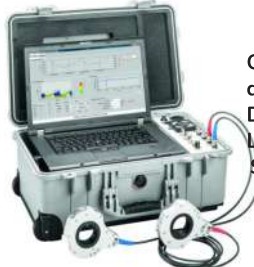
Online Partial discharge Diagnostics Liona: Online PD Spot Tester
