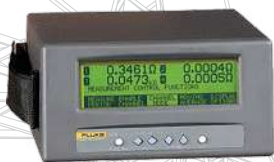
1529 Chub-E4 Standards Thermometer
