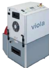
Portable VLF testing and tan delta Diagnostics Frida TD: High-voltage testing and diagnostics device. Viola TD
