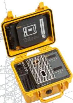
9009 Industrial Dual-Block Thermometer Calibrator (Field dry-block calibrators)
