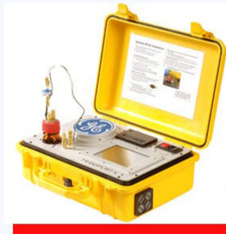
TRANSPORT X-A Portable DGA
