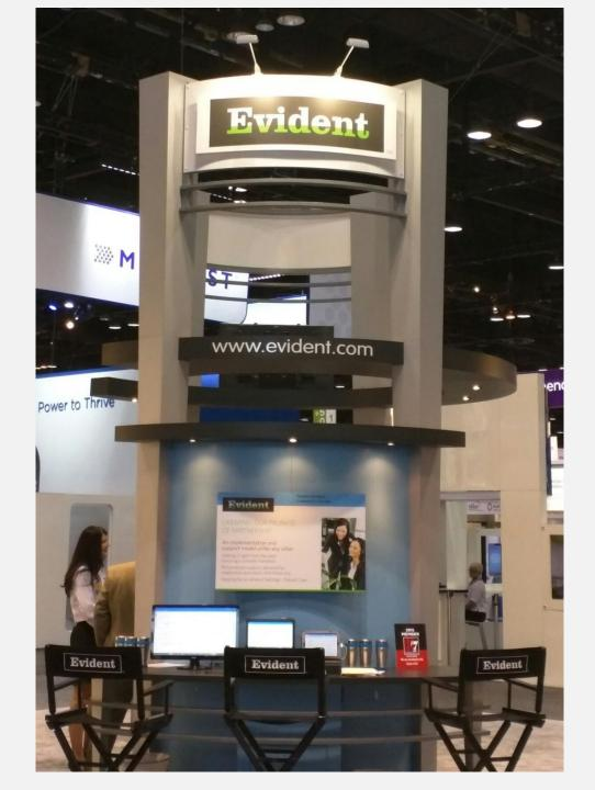
LED illumination of perimeter tension fabric structure. Color corrected white T5 fluorescent light inside of hanging tension fabric pendants.
