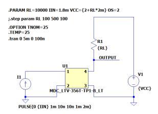
.meas tr TRIG V(output)= $\{VCC-\{OS\}\}$ \*0.9+ $\{OS\}$  FALL=2 TARG V(output)= $\{VCC-\{OS\}\}$ \*0.1+ $\{OS\}$  FALL=2 .meas tff TRIG V(OUTPUT)= $\{VCC-\{OS\}\}$ \*0.1+ $\{OS\}$  RISE=2 TARG V(OUTPUT)= $\{VCC-\{OS\}\}$ \*0.9+ $\{OS\}$  RISE=2 .meas td FROM 3m TARG V(output)= $\{VCC-\{OS\}\}$ \*0.9+ $\{OS\}$  FALL=2 .meas ts FROM 4m TARG V(output)= $\{VCC-\{OS\}\}$ \*0.1+ $\{OS\}$  RISE=2
