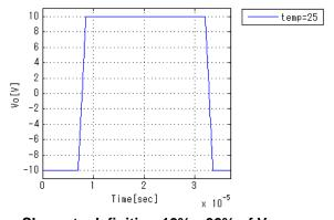
Slew rate definition:10%  $\sim$  90% of  $\rm V_{\rm O}$
