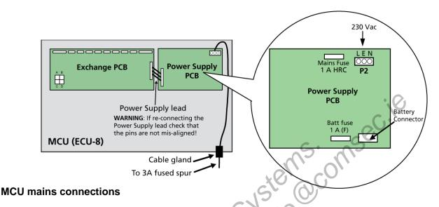
The MCU requires fixed wiring using 3-core cable (no less than 0.75 mm² and no more than 2.5 mm²) fed from an isolating un-switched fused spur, fused at 3 amps and must not be connected using a plug and socket. The 230 VAC cable MUST enter the enclosure via one of the inlets at the bottom right hand corner of the enclosure. Ensure that mains cables are kept as far away as possible from all other cables.
