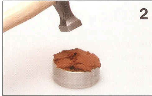
2. Fill the ring with Delft Clay. Compact clay with a hammer.
