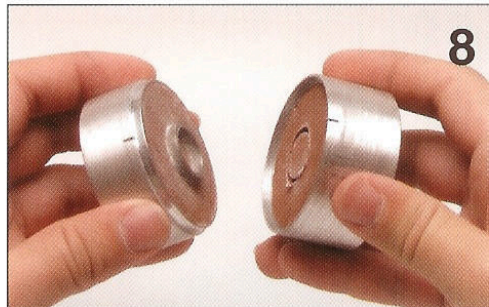
8. Remember to keep the position of the aligning marks together. Replace the rings later in the same position. Separate the rings.
