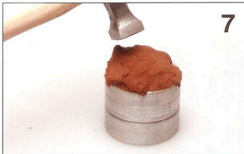
7. Fill the second ring with clay. Compact it with a hammer. Remove excess clay with a ruler.
