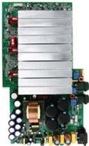
High current components & FR4 fire retardant circuit card
