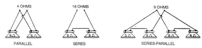
The actual formula for calculating parallel impedances is Z parallel =  $\frac{1}{Z_1} + \frac{1}{Z_2} + \frac{1}{Z_3} + \dots + \frac{1}{Z_n}$ The formula for series impedance is Z series =  $Z_1 + Z_2 + Z_3 + \dots + Z_n$
