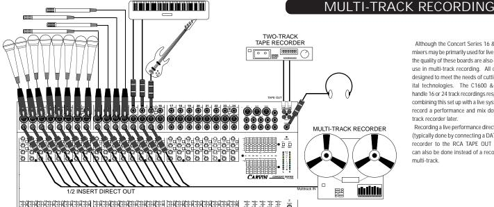
Although the Concert Series 16 & 24 channel mixers may be primarily used for live applications, the quality of these boards are also designed for use in multi-track recording. All channels are designed to meet the needs of cutting edge digital technologies. The C1600 & C2400 can handle 16 or 24 track recordings respectively. By combining this set up with a live system, you can record a performance and mix down to a two track recorder later.
