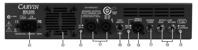
LEVEL control. This output is controlled by the MUTE function so you may tune your bass quietly while using the MUTE. The DIRECT OUT signal is not affected by the MASTER level. TONE controls. 9-band EQ or effects loop. The XLR is protected against Phantom power (DC voltage) on cables coming from phantom powered mixer inputs.
