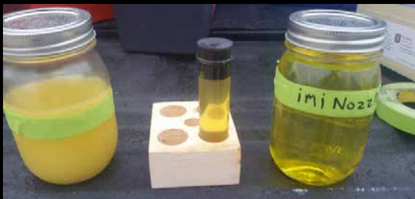
Left side: Carboxylates in diesel fuel. Right side: Klenz ID ® , at quick clean dose, took care of the carboxylates and cleared up the diesel fuel.
