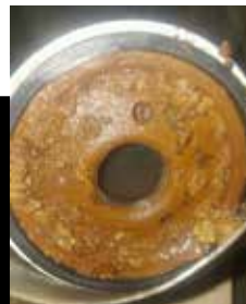
Corroding filter housing caused by carboxylates / sticky IDID.
