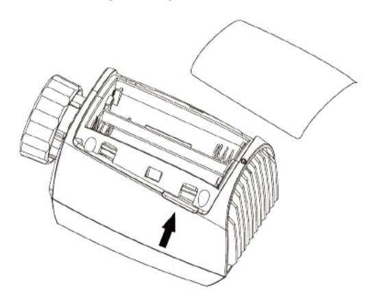
The service life of new alkaline batteries is approximately 1.5 years. A battery symbol ( LRL ) on the display indicates that the batteries need to be replaced. After removing the empty batteries, wait approx. 1 minute before inserting the new ones. This device does not support operation with rechargeable batteries.
