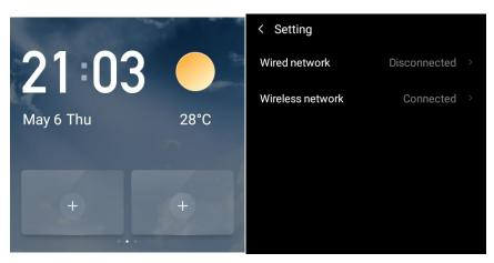
(2) There are two options in the network settings. You can select wireless connection or wire connection. There will be a QR codeshowing on the screen after the network connection is done.
