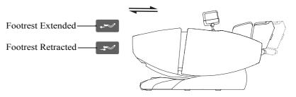
▶ A footrest sensor is set at the bottom of footrest the footrest will adjust the length automatically once the chair started.
