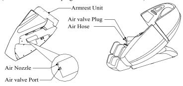
▶ Hold the armrest unit up and hook the hanger 2 onto the carrier groove, slowly push the armrest unit back into the chair linkage until hanger 2 aligns completely with hanger 4, insert hanger 1 into hanger 3, use a screw to secure the armrest into place. (Same installation method with the other side)
