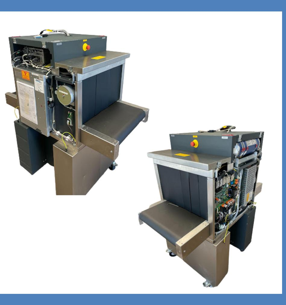
With both side panels removed, you can move on to removing the front curtain cover.
