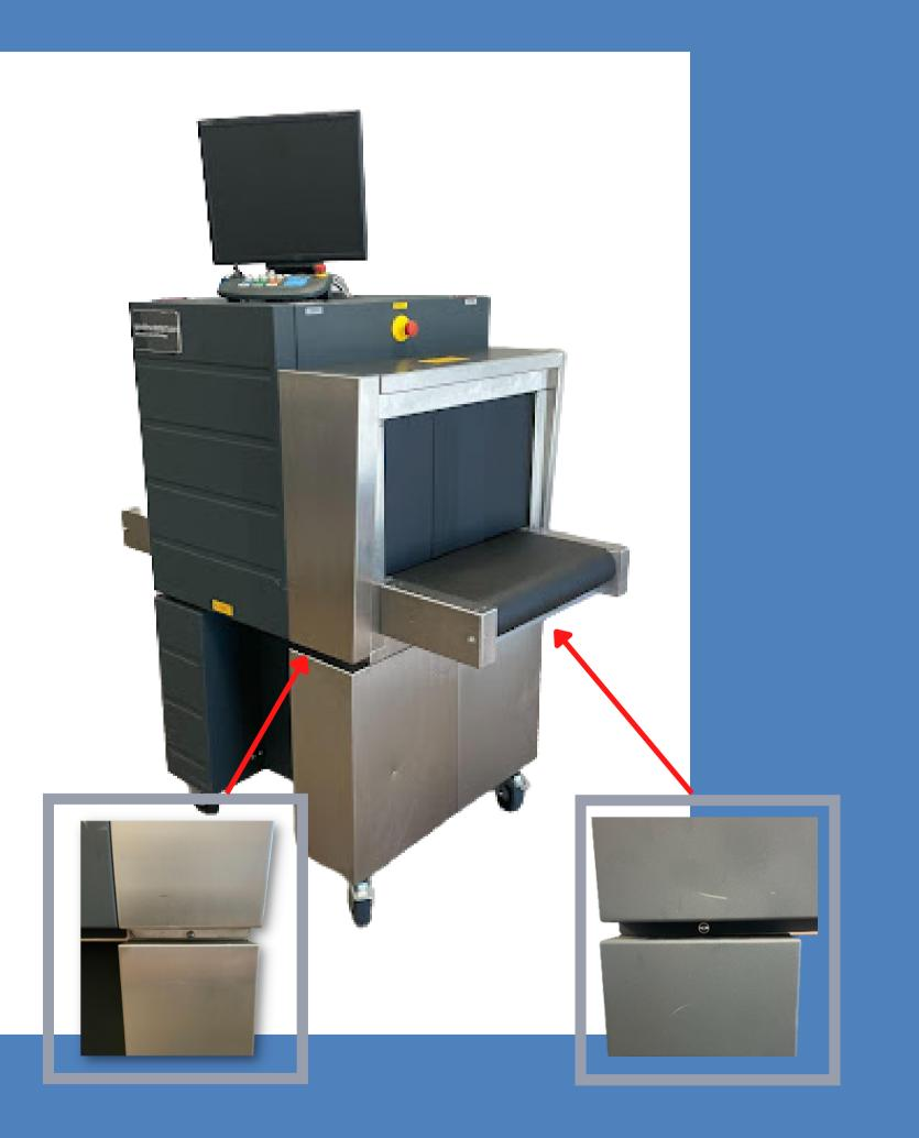
With all external components disconnected, locate the two screws holding the left side panel in place and, using a 3mm hex key or bit, remove and set them aside.
