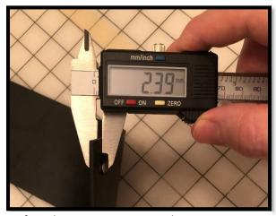
3. If you have a micrometer, take a measurement or the curtain thickness. This helps us confirm you have the correct radiation protection level.
