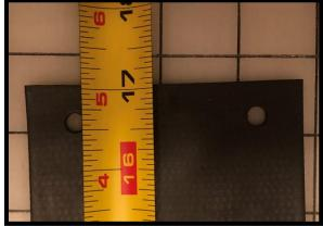
1. Measure the curtain lengthwise. Ensure the hangar holes are visible when you take a picture.
