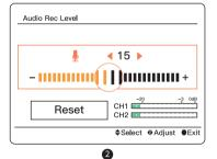
Adjust the recording level of inbuilt mics for Canon Camera (Take EOS 5D Mark IV for example)
