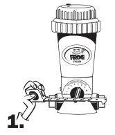
Measure the distance between POOL FROG\* Cycler male adapters and cut out a section of pipe 3" less than that dimension.
