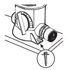
Use Phillips pan head screws through the mounting holes at the POOL FROG® Cycler base to secure the POOL FROG® Cycler into a treated wood base.
