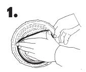
Hold cap in front of you upside down with the o-ring groove facing up. Place one end of o-ring into cap groove at the point closest to you. Hold o-ring down with the thumb and index finger of one hand.
