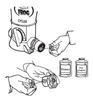
Following Primer directions, brush Primer on reducer bushings and inside of male adapters. Repeat this process with PVC cement following directions on that product.
