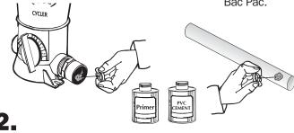
Following Primer directions, brush Primer on the inside of the male adapters and to ends of pipe. Repeat this process with PVC cement following directions on that product.
