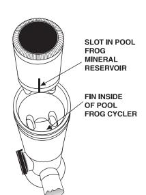
Find slot on side of POOL FROG® Mineral Reservoir and line up with fin inside the POOL FROG® Cycler. Lower POOL FROG® Mineral Reservoir into POOL FROG® Cycler until secure.
