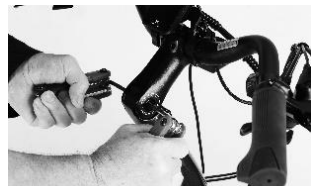
Adjust stem angle and re-tighten the bolt under the stem and the two side bolts.
