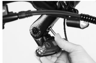
Undo bolt underneath stem \frac{3}{4} of a turn
