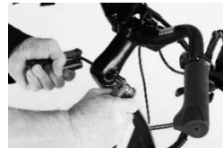
Undo center bolts on both sides
