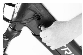
Locking after battery insertion
