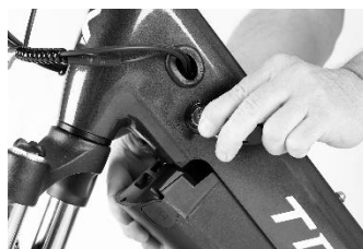
Pushing battery up & unlocking
