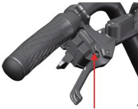
Fine adjustment bolt / 2mm Allen wrench
