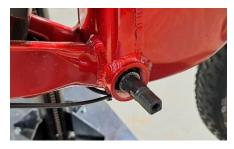
2. Once the right-side cup is removed, slide the B.B. set out from the right side of the bike and be careful not to damage the wire. Pull the B.B. set out with its wire attached and unplug it at the connection with the main wire harness as it comes out. You can now fully remove the B.B. set on that right side (see below). Remove the left side cup <u>only if needed</u> by unthreading it counterclockwise.
