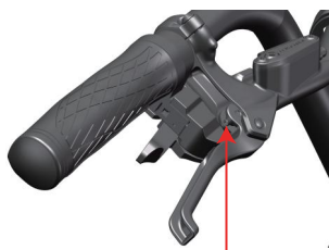
Fine adjustment bolt / 2mm Allen wrench
