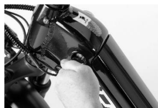
Lock battery in frame
