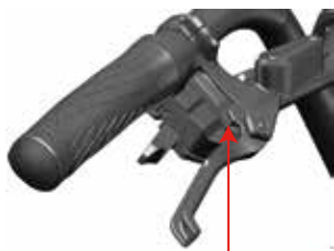
Fine adjustment bolt / 2mm Allen wrench
