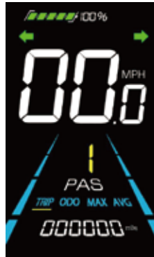
Hazard Lights function selected
