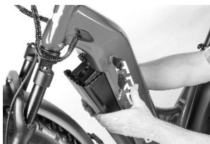
Pushing battery up (unlocked)
