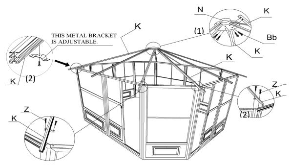
**Note:** Do not tighten the bolts right away as you may have to adjust the angle when inserting the PC roof panels.
