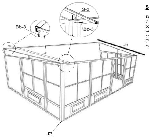
Set left rafter F over last bracket then secure it with Bb-3 screw and continue screwing through joint K-3 with the Bb-3 screw. Secure to Q-3 bracket with self-tapping screw (PQ-3). Repeat on right side with rafter F1.
