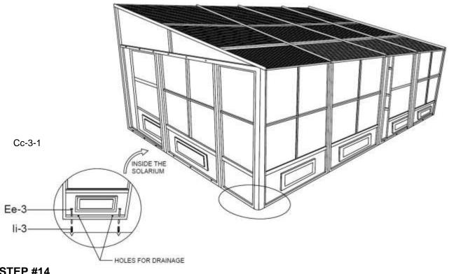
Anchor the solarium to the deck or floor securely using screws and shields supplied. See diagram below.
