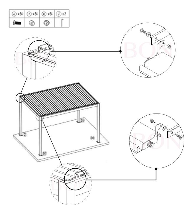
Mark holes for expansion bolt <sup>(1)</sup>x4 on each post.
