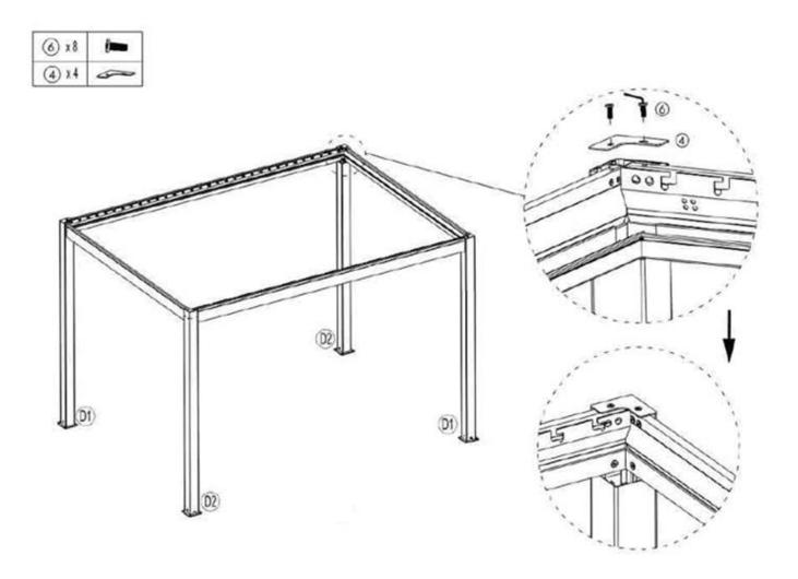
1. Slide the 9 motor into F gutter before hooking onto the beam in the direction as shown below.
