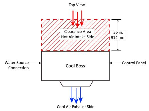
2. Keep 36" / 914 mm minimum behind the Cool Boss open for air intake.
