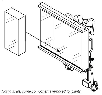
6. Install the Media Splash Guard using the three screws removed in step 1.
