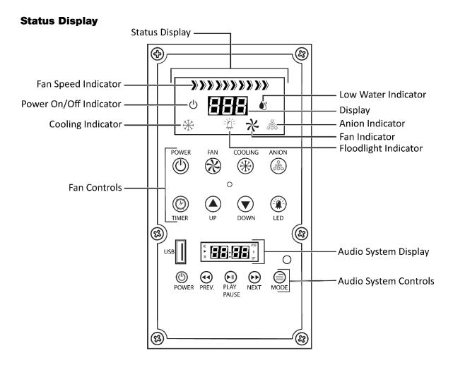
The Control Panel's Status Display provides the on-off status of the Cool Boss functions, the fan power settings as a percentage, current temperature of the air in °F at the Cool Boss Fan, the timer status and a low water warning.
