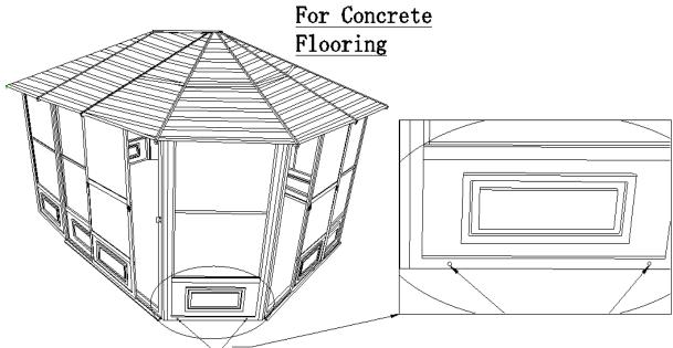
On the outside face, it is suggested to drill holes at the bottom end of the panels to permit drainage when installing on Concrete floor
