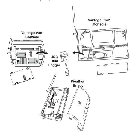
6. Insert the serial data logger. Press into place FIRMLY.
