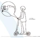
5. Continuously press the throttle to speed up.
