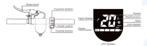
**Power Switch:** Press and hold the power button to turn on/off.
